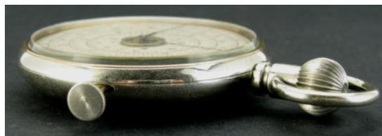
The winder angle is very different ( $75^\circ$ ) versus  $30^\circ$  or  $25^\circ$  for the HC or FC Calculigraphe clutch respectively, or  $27^\circ$  for the Queen example. The mechanism is also completely different to any known example from any of the makers we have shown here, e.g. the very prominent central axle.
