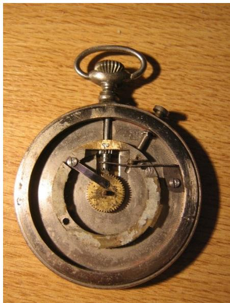
The mechanism at left is that of a “thin” Calculigraphe, as evidenced by the furniture. However, by careful study we can guess that it is perhaps yet another anomalous type because it has three equally spaced fixing screw holes on the fixed annulus of the body, something not seen on any of the identified “thin” types so far listed.
