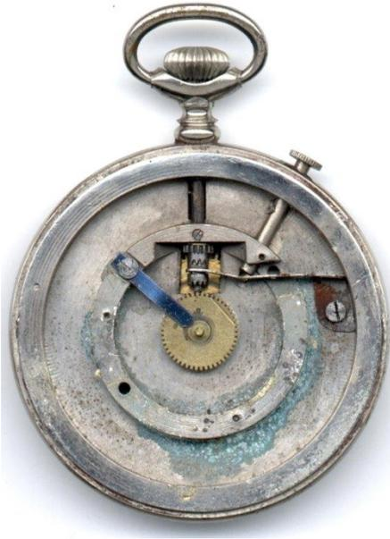
*Thin calculigraphe mechanism- front*
