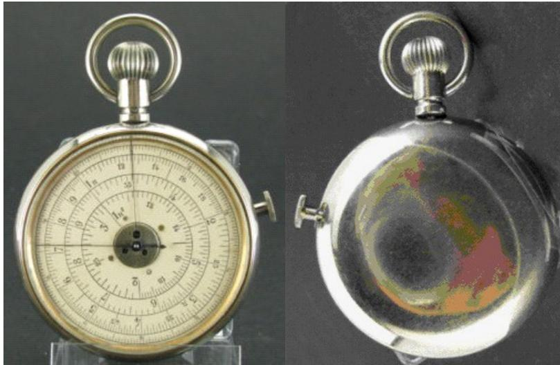
And then where would this device fit? Sold on eBay in Dec 2013, it is probably the only so far known example of a single sided Calculigraphe – the button appears more like a clutch than a winder – and the single scale is a ‘normal’ rotating scale as on any other two-sided Calculigraphe. But it is completely different to the single-sided, single-scaled Calculigraphe illustrated in *La Science Illustrée* edition No 347 of July 1894, see Appendix B.
