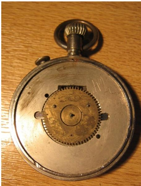
Minor detail differences between fat and thin devices are also obvious. The thin device uses a tiny grub screw in the top of the annulus to hold in the crown axle, the fat device uses a separate spring which locates in thin shallow rings in the crown axle and also the push button clutch for location. This is a more expensive but probably ultimately a smoother solution.
