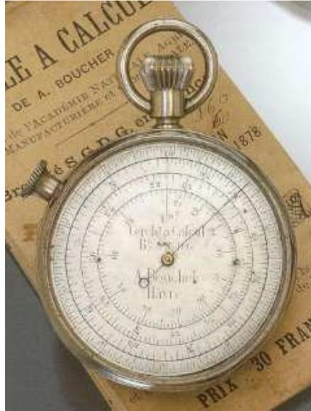
The second example is the one previously covered which was part of a MAF Boucher Calculator and is repeated here for completeness.
