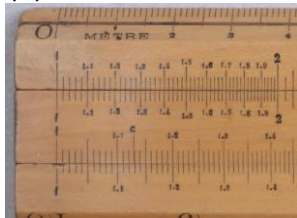
Plain scales, decimal notation, hand printed numbers typeface A, displaced 1.5
