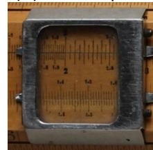
Nickel plated brass, chisels, 2 mm adjusting screws, rounded window, no spring
