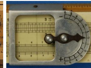
Aluminium, digit registering with 2 domed rivets, rounded window, centre riveted spring
